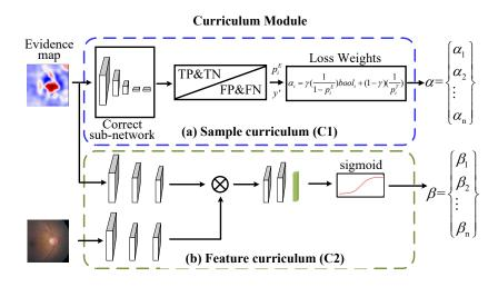
Fig. 4: The dual-curriculum adaptively provides two types of weights  $\alpha$  and  $\beta$  along with the training procedure as the sample curriculum (a) and feature curriculum (b), respectively. The weights  $\alpha$  and  $\beta$  are adopted in teacher network to balance the training benefits for unbiased glaucoma diagnosis.
